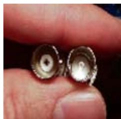
For SPDIF ideally 75 ohm connectors are used to minimize "reflections" of the signal (which can, if large enough, introduce sound quality robbing jitter errors). We consider it important to maintain a 75 ohm connection all the way thru the signal path which includes the jacks, plugs and cable.
